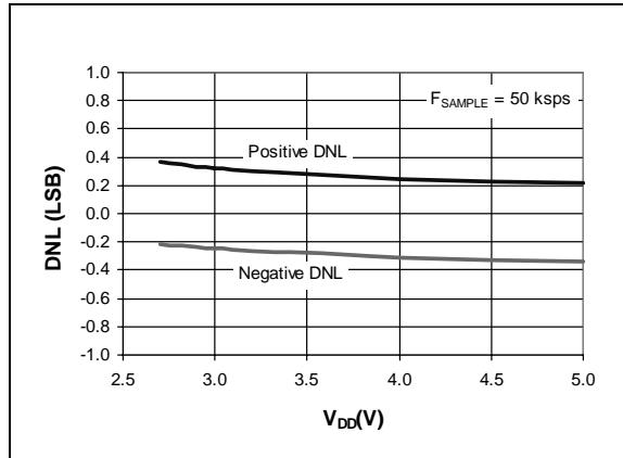
**FIGURE 2-12:** Differential Nonlinearity (DNL) vs.  $V_{DD}$ .
