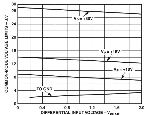
Figure 17. Input Common-Mode Range for Single Supply
