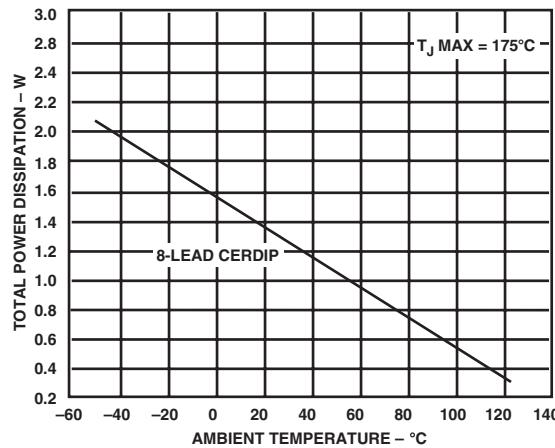
Figure 4. Maximum Power Dissipation vs. Temperature, CERDIP Package
