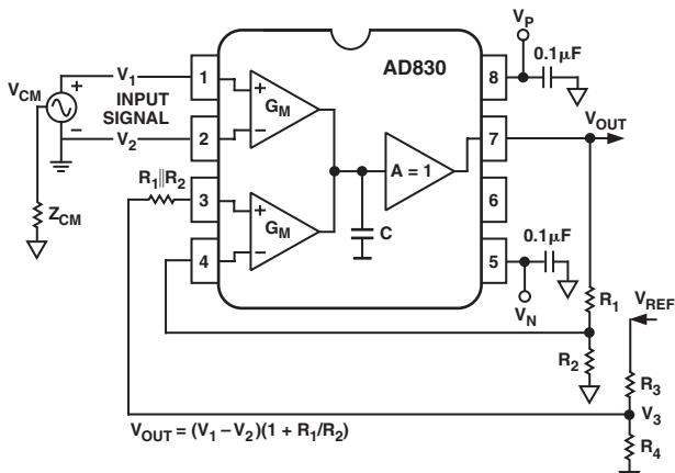
Figure 22. Offsetting the Output with Differential Gain  $> 1$
