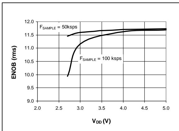
**FIGURE 2-25:** Effective Number of Bits (ENOB) vs.  $V_{DD}$ .
