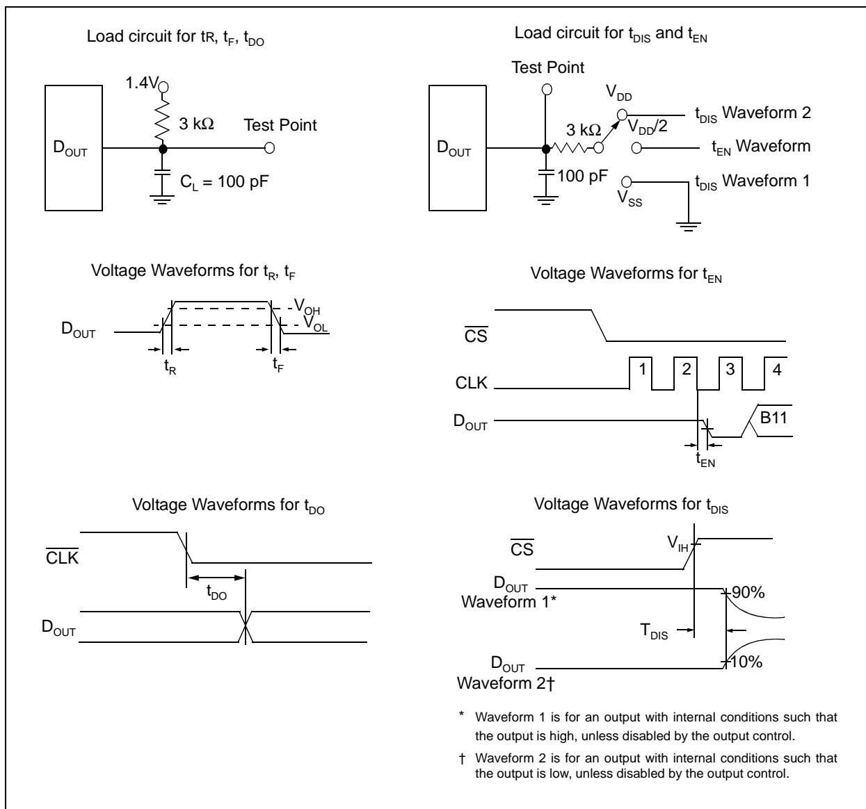
FIGURE 1-2: Test Circuits.
