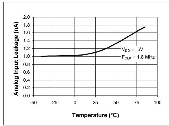
FIGURE 2-36: Analog Input leakage current vs. Temperature.
