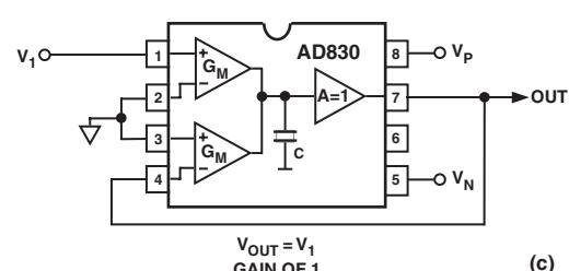
(c)  $V_{\text{OUT}} = V_1$
