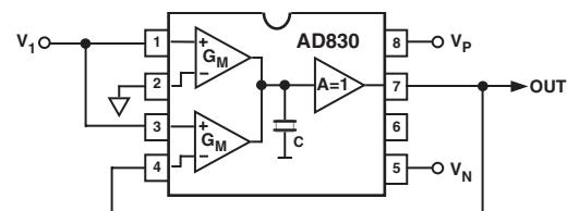
(a)  $V_{\text{OUT}} = 2V_1$
