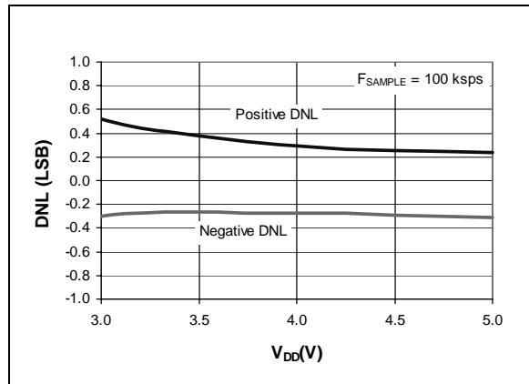
**FIGURE 2-9:** Differential Nonlinearity (DNL) vs.  $V_{DD}$ .
