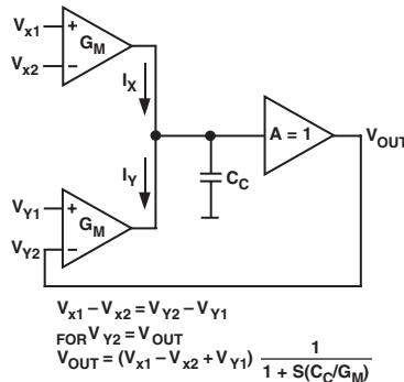
Figure 8. Closed-Loop Connection
