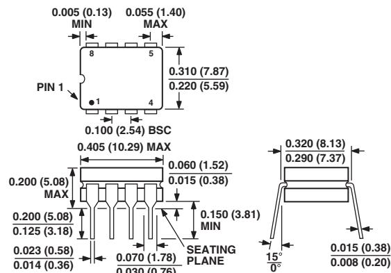
**CONTROLLING DIMENSIONS ARE IN INCHES; MILLIMETERS DIMENSIONS
