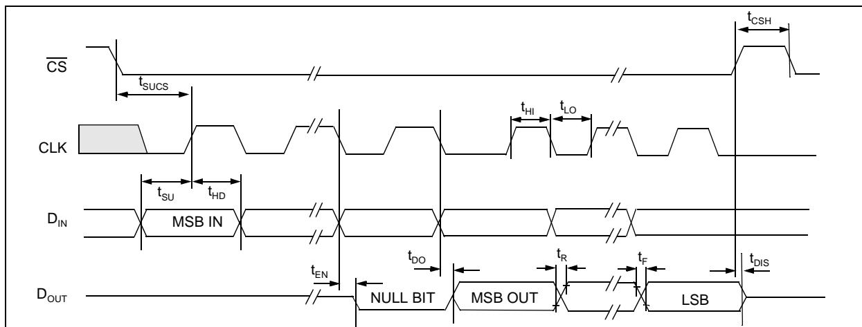
FIGURE 1-1: Serial Timing.
