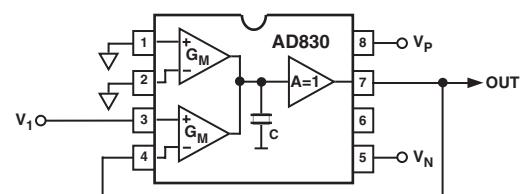
(b)  $V_{\text{OUT}} = V_1$
