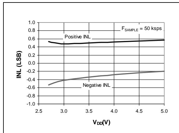
**FIGURE 2-5:** Integral Nonlinearity (INL) vs.  $V_{DD}$ .
