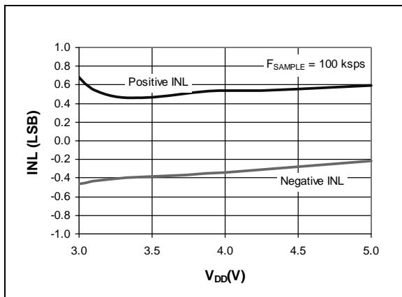
**FIGURE 2-2:** Integral Nonlinearity (INL) vs.  $V_{DD}$ .
