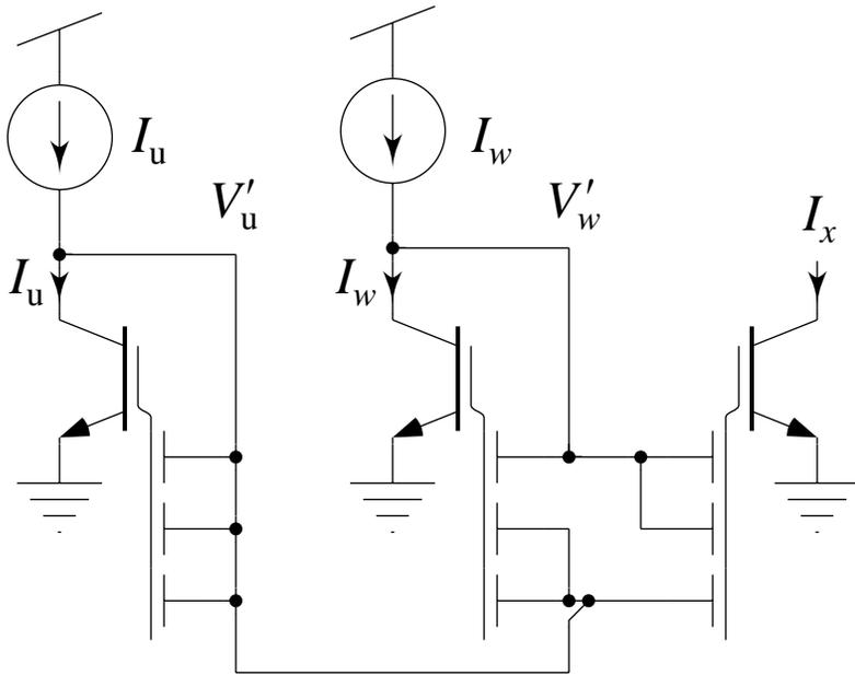
⇒ We can connect  $V'_u$  and  $V'$  together without changing the function of the MITE network...
