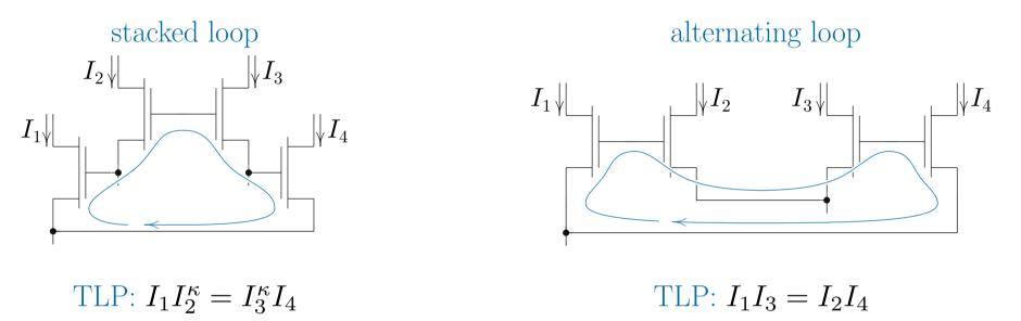
This restriction does not limit the class of systems that we can implement. However, designs based on alternating loops generally consume more current but operate on a lower power supply voltage than do designs based on stacked loops.
